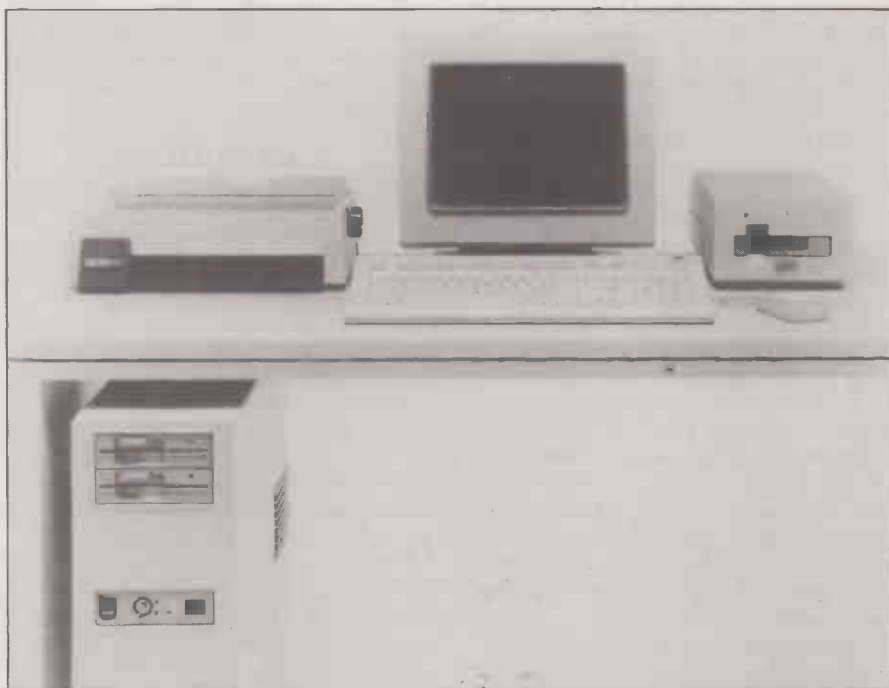
Both the floor-standing 6150 (above) and the desk-top 6151 (below) run IBM's new Risc technology chip.
